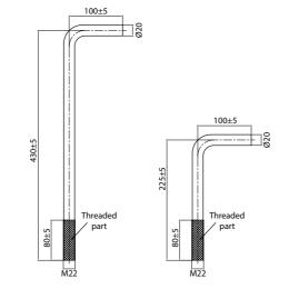
Fig. 4. Anchor bolts used to mount structure in foundation
