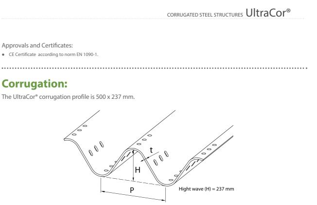
Fig. 1. Wave profile of UC plate
