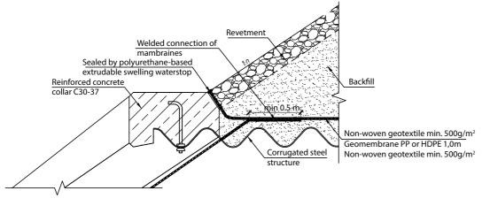
Fig 11. Detail of concrete collar with drip
