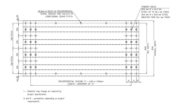
Fig. 3. Geometry of UltraCor plate.
