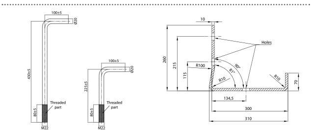
Fig. 5. Base channel used to connect structure to foundation.
