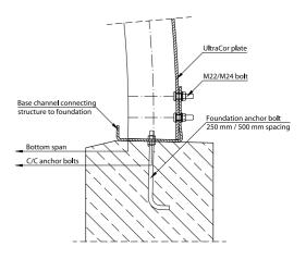
Fig. 9. Connection of UltraCor® structure with concrete footing
