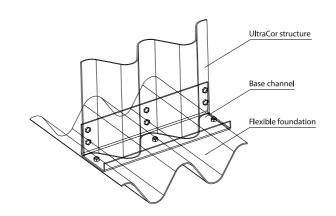
Fig. 8. Connection of UltraCor® structure with flexible footing
