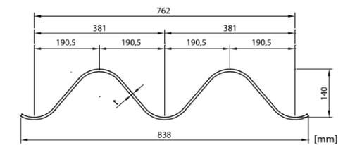
Fig. 2. Cross section of SuperCor® plate
