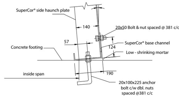
Fig. 10. Connection of SuperCor® structure with concrete footing
