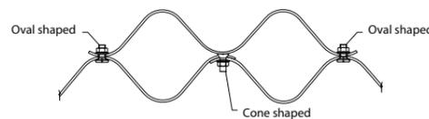
Fig. 5. Connection of ribs to main barrel plates
