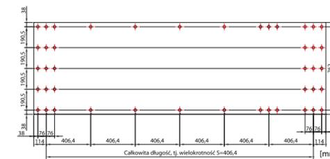
Fig. 1. Geometry of SuperCor® plate (total length, i.e. multiple S=406,4 mm)
