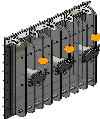
3D image of an arrangement for 3 smaller pet flaps in one larger flap.
